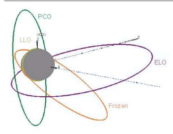
Low Lunar Orbit (LLO): LLO is defined as a circular orbit of an altitude around 100 km. LLOs are favorable for surface access and polar orbit inclinations offer global landing site access.
